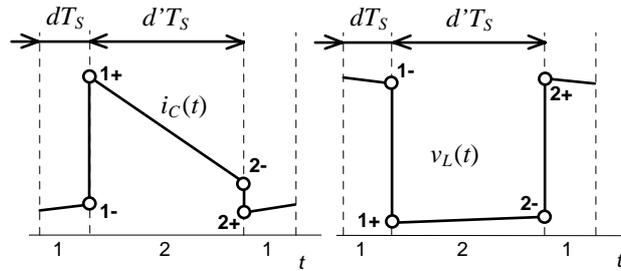
Fig. 2: Piece-wise approximation of time derivatives of converter state variables.
